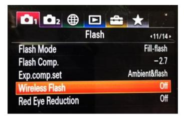
In this Manual Mode the **flash intensity manual adjustment by camera menu** also becomes available. Pay attention, underwater strobe must be in STTL mode for this function. Then, user can comfortably adjust flash intensity by camera wheel, looking at the camera scale. Full scale range (-3ev....+3ev) corresponds to flash intensities 1/64 ...1/1.
