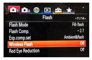
In this Manual Mode the **flash intensity manual adjustment by camera menu** also becomes available. Pay attention, underwater strobe must be in STTL mode for this function. Then, user can comfortably adjust flash intensity by camera wheel, looking at the camera scale. Full scale range (-3ev....+3ev) corresponds to flash intensities 1/64 ...1/1.
