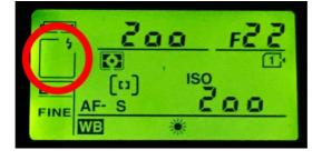
• If "Flash" symbol does not appear on the screen, it means that intellectual communication protocol between camera and TTL Converterdoes does not work.
