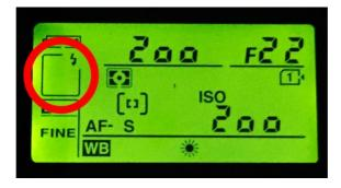
• If "Flash" symbol does not appear on the screen, it means that intellectual communication protocol between camera and TTL Converterdoes does not work.
