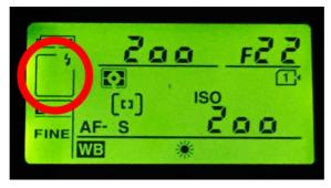
If "Flash" symbol does not appear on the screen, it means that intellectual communication protocol between camera and TTL Converter does not work.
