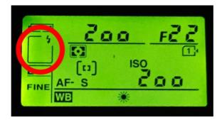
• If "Flash" symbol does not appear on the screen, it means that intellectual communication protocol between camera and TTL Converterdoes does not work.
