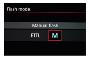
In such Manual mode also becomes available flash output level scale in submenu. User can adjust flash output level by camera wheel, looking to this menu scale (or looking to camera service screen):
