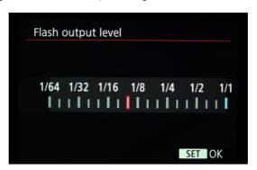
Some manual underwater strobes (like MF-1) requires very strong optical signal for synchronization, this case necessary to set maximum power by this scale (1/1).
