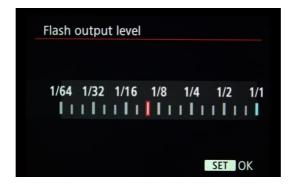
Some manual underwater strobes (like MF-1) requires very strong optical signal for synchronization, this case necessary to set maximum power by this scale (1/1).
