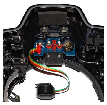
• Remove the mirror prism and its plastic podium from the housing. In the modern Nauticam housings it is easy to make by unscrewing just 1 or 2 bolts. In the Nauticam housings of former years it was necessary to use a sharp knife to pick up mirror prism and remove it from the podium, then unscrew 2 bolts of the podium. (Prism was glued very slightly like a sticker on the plastic podium, it was easy to remove it by the knife).
